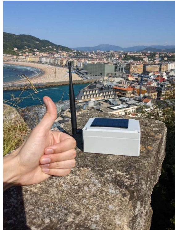
Embedded solar panel powered Isurlog Compact LoRa outpost at the Urgull mountain in San Sebastian (Spain), linked to ISURKI's headquarters based LoRaWAN gateway through 13 km of hilly terrain. ↑ ↓
